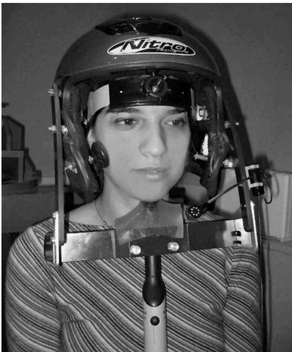
FIG. 19.7. Ultrasound probe fixed beneath a subject's chin, by means of a holder attached to a helmet, for the collection of speech data. The head of the probe is covered with a sheet of jelly-like material, which aids efficient transmission of the signal.
